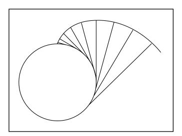
Involute gear tooth forms and standard tooth proportions are specified in terms of a basic rack which has straight-sided teeth, for involute systems.
